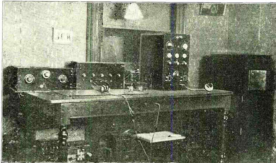
The Receiver of This Station is One of the Three-circuit Regenerative Variety, Employed With Four Stages of Audio Frequency Amplification. The C.W. Set is Seen at the Extreme Right. Phone is Used for Local Work.
